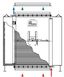
Packman Co. offers an extensive selection of boiler economizers specifically designed to recover the lost heat exiting from exhaust stacks and preheat water. Our broad line of economizers covers the spectrum of boiler sizes, ranging from very small hot water boilers with burner inputs of 1000 Kw to large boilers delivering steam at 32.000 Kg/h and greater.
